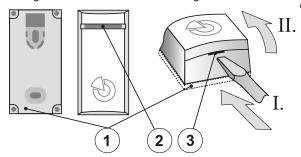
Figure 1: 1 - separation plate; 2 - red activation indicator; 3 - cover tab
