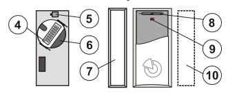
Figure 3: 4 – production code; 5 – tamper contact; 6 – battery; 7 – permanent magnet; 8 – magnetic sensor; 9 – red detector activation indicator; 10 – alternative location of the permanent magnet
