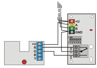
Figure: example of a connection enabling dual-colour indication of the PG output status
