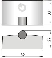
Figure: the JA-111I indicator dimensions.
